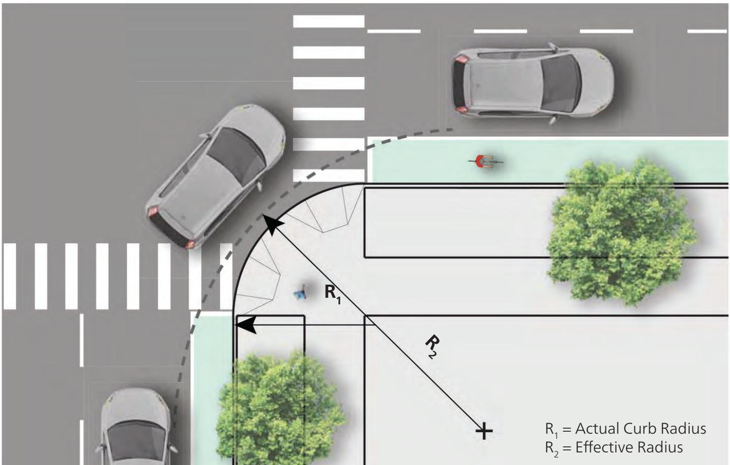
Reduce curb returns on urban typologies to ensure safer crosswalk design and reduce crossing distances
